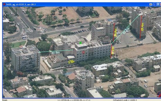
**Figure 5.** Height and distance measurements (Aeromap, 2006)
