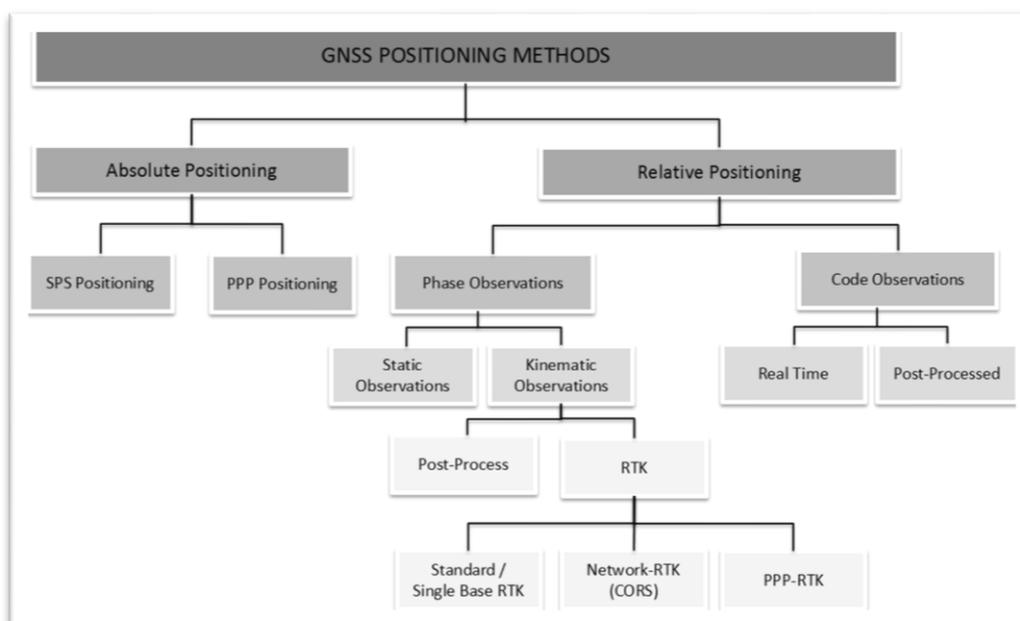
**Fig. 1.** General Classification of GNSS Positioning Methods
